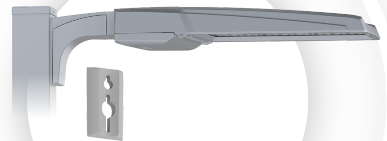
'SPM' Square & 'RPM' Round Pole Arm Mount can retrofit up to 5-1/4" max bolt spacing (allows for single person installation)
