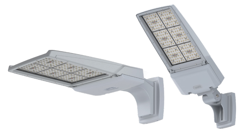
'WM' Wall Mount Recessed J-Box Installation 'AWM' Adjustable Wall Mount Recessed J-Box direct mounts to 3" & 4" square/octagonal recessed J-box (J-box provided by others)
