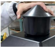
2. Place the cupola on top of the photocell and rotate so the photocontrol window is centered in the cupola window.
