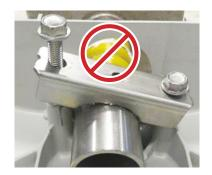
WARNING: Avoid tightening bolts unevenly, as it may cause cross-threading.
