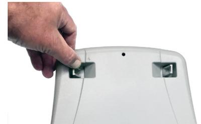
**Step 3** Loosen the slip-fitter bracket bolts and insert the mounting arm. The maximum outside diameter for the mounting arm is 2-3/8" (60.3mm). The minimum outside diameter for the mounting arm is 1-5/8" (41.28mm). Mounting arm to be placed "stopped" against appropriate step required to achieve desired degree of tilt. Steps vary from from 0° to get no tilt to the options shown below.
