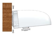
After wiring, the luminaire is simply hung from the top of the back plate and secured with inset, discreet set screws. Eseta is IP66-Rated, so no sealant is needed.
