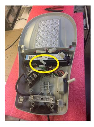
**Step 4** - Connect the dimming leads found in step 3 to the power supply dimming leads. Purple wire from the PCR7 receptacle to purple wire from the power supply. Gray color wire from PCR7 receptacle to gray color wire from the power supply.
