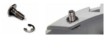
Captive screws are attached to each corner of the 80 Degree Cutoff Shield to align with the threaded holes in the fixture's housing. Place the shield on the underside of the light fixture as shown and firmly tighten the screws.
