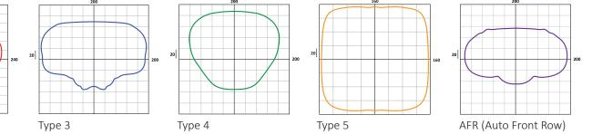
Micro-lens Optics produce IES Type 2, Type 3, Type 4, Type 5 distributions for Roadway and Area lighting applications. Factory rotated optics can be ordered for special applications.
