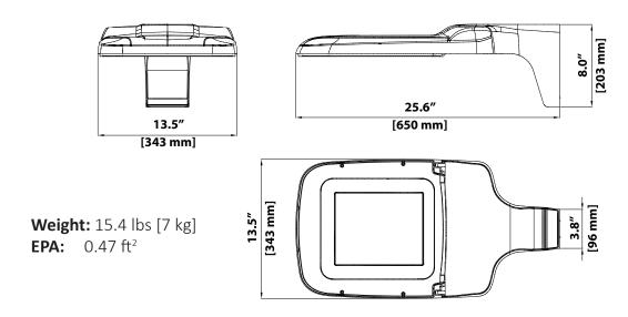
Please review the ComfortGuide™ Specification Data Sheet available for download at Leotek.com for complete photometric capabilities and features.
