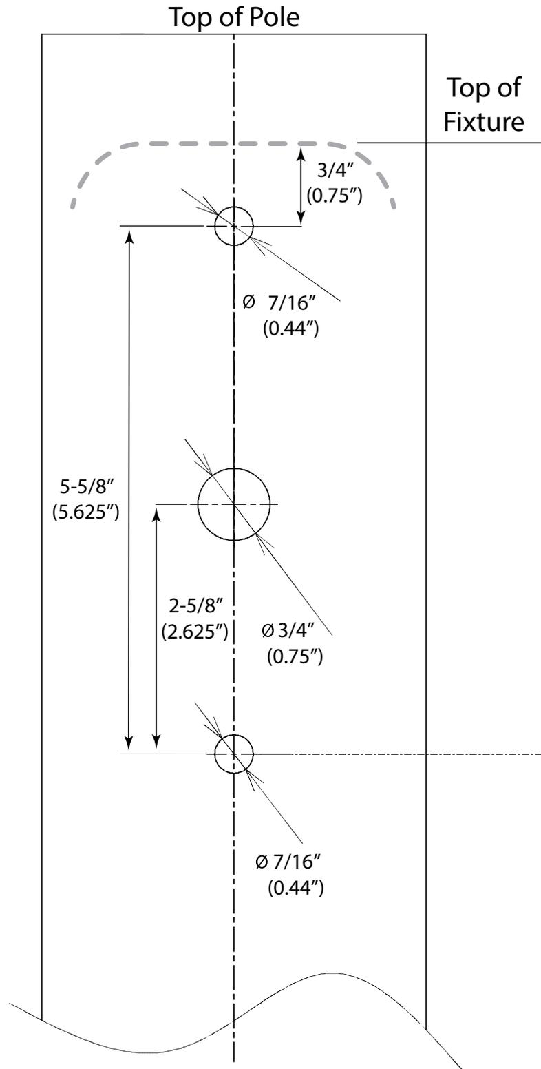
**Mounting Pole Drilling Dimensions
