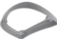
80 Degree Cutoff Shield mitigates high angle glare above 80 degrees from nadir and cuts light off at 1½ times the mounting height behind and 2¼ times the mounting height laterally.
