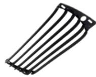
Flush mounted House Side Shield cuts light off at 1 times the mounting height behind the luminaire and 2¼ times the mounting height laterally.
