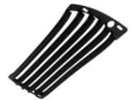
Flush mounted Front Side Shield cuts light off at approximately 1½ times the mounting height in front of the luminaire (street side) and 2¼ times the mounting height laterally.
