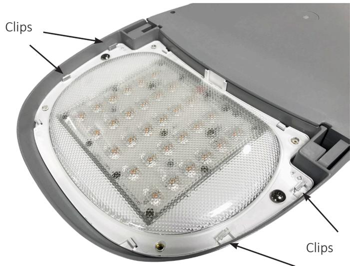
Place the shield so that the slots align with the clips along the edge of the ComfortView Light Engine, then simply push the edges of the shield down to clip it into place.
