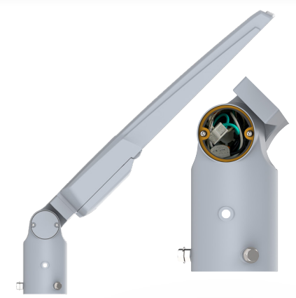
'SF' Slipfitter #1 w/ available wire leads located inside UL splice compartment (compatible w/ 1-5/8", 2-3/8" & 3" O.D. tenons, pre-aimed @ 45° tilt option available)
