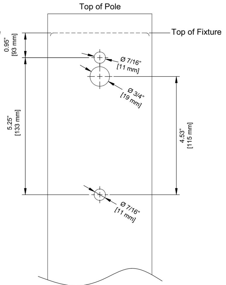
New Construction Pole Mount Drilling Dimensions
