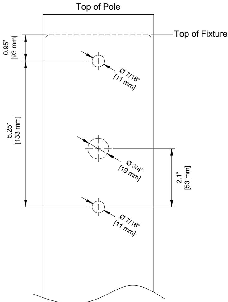
New Construction Pole Mount Drilling Dimensions
