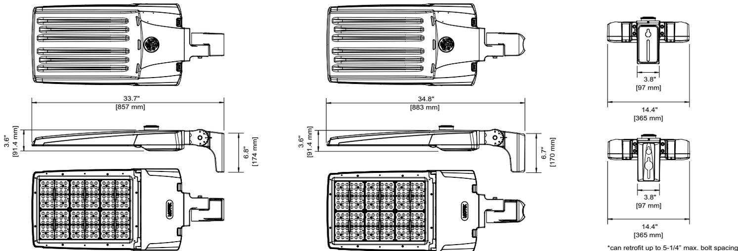
\*can retrofit up to 5-1/4" max. bolt spacing
