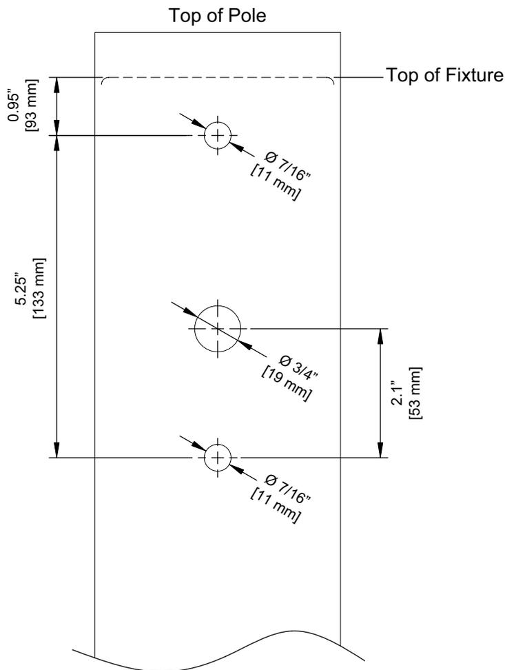
New Construction Pole Mount Drilling Dimensions
