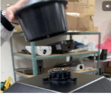
1. If optional 6 position cupola is ordered (“C” accessory code), and optional receptacle (“PCR7-CR” option code), rotate the photocell receptacle on top of the luminaire until the indicator points north. Install the photocontrol and lock in place
