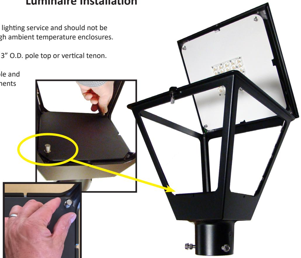
**Step 3** - Feed service lead wires through bottom of fitter into wiring compartment. Place fixture on pole top (care must be taken not to pinch service leads). For fixture with asymmetric light pattern (Type 2,3), locate the word "Street side" on the housing overhang. Position fixture on pole so "Street side" faces the street.
