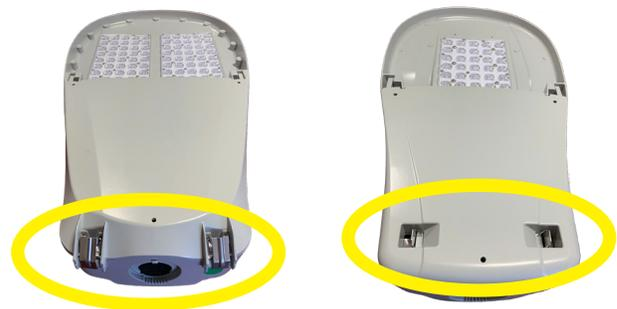
**Step 3** Loosen the slip-fitter bracket bolts and insert the mounting arm. The maximum outside diameter for the mounting arm is 2-3/8" (60.3mm). The minimum outside diameter for the mounting arm is 1-5/8" (41.28mm). Mounting arm to be placed "stopped" against appropriate step required to achieve desired degree of tilt. Steps vary from from 0° to get no tilt to the options shown below.
