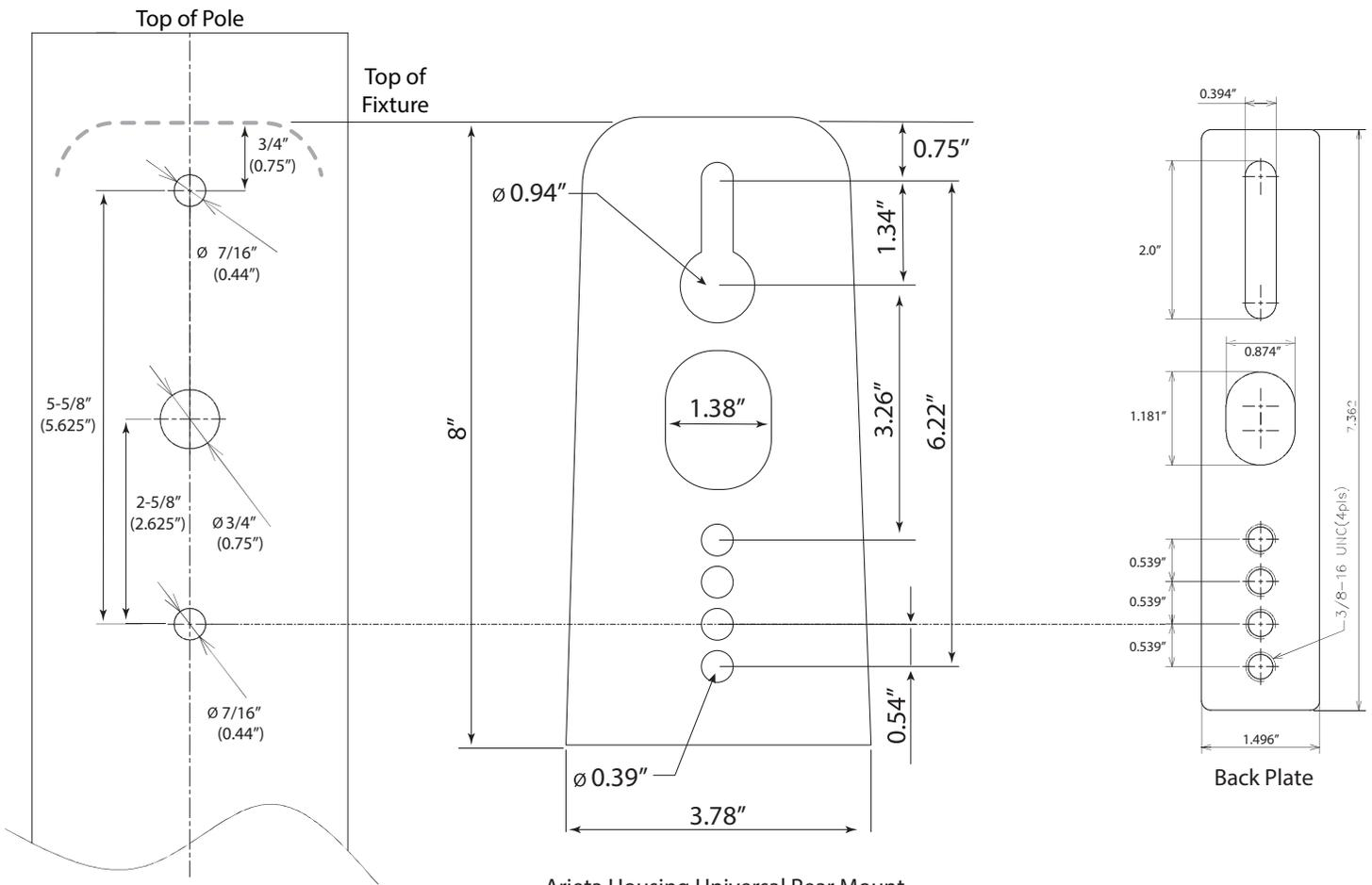
Mounting Pole Drilling Dimensions for New Construction
