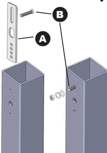
**Step 1** - Install the back plate **A**
