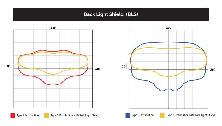
The Arieta Back Light Shield replaces the standard Arieta bottom plate cover. Simply remove the original bottom plate cover and replace it with the Back Light Shield utilizing the same 8 screws.
